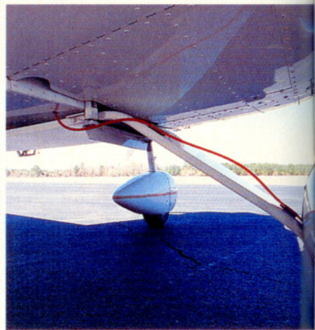
The somewhat utilitarian interior includes sturdy, high-G seats and a small cargo shelf. The single-piece main landing gear and exposed brake line emphasize function over form.
